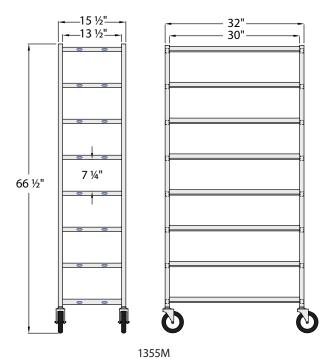
The ideal transport/storage rack for the meat department. These racks accommodate platter sizes from 10"x 30" to 12" x 30". The unique radius of the oval tubing shelf design allows for easy on, easy off access to platters.
