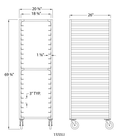
MATERIAL: Heavy duty, high tensile, extruded aluminum. Type 6063-T5 alloy. Extruded on site.
