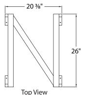
**MATERIAL:** Heavy duty, high tensile, extruded aluminum. Type 6063-T5 alloy. Extruded on site.
